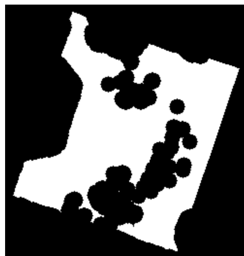
Figure 3: Binary costmap generated by thresholding the Nav2 costmap into free and occupied space.
